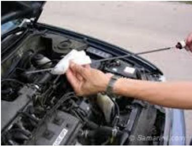
You can check automatic transmission fluid with the dipstick (*on older cars. The newer ones have a sealed system*), usually located at the back of the engine. The dipstick itself will be a different color than the oil one. Fords usually have a red one, as the fluid is red.
