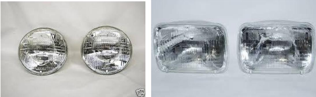
To change these, you will need a screwdriver to loosen the framing around them in the front, outside of the car. Then pull the plug out from behind the bulb. Put a new bulb inside the framing, plug it in, and align the frame to the holes and put the screws in.
